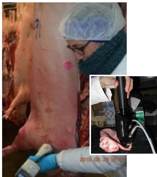
*New technologies have shown promise in assessing meat quality. Left: Using a spectrophotometer to assess bruising colour. Right: Using NIRS on pig ears. Photos: AAFC*
